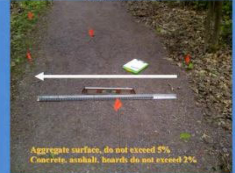
Figure 2: Measuring Cross Slope of an accessible trail. © photo 2013 Penn Trails LLC
