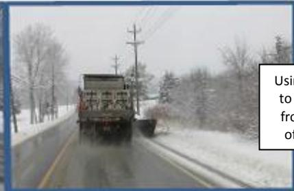
Using the wing plow to push back snow from the shoulder of the roadways.
